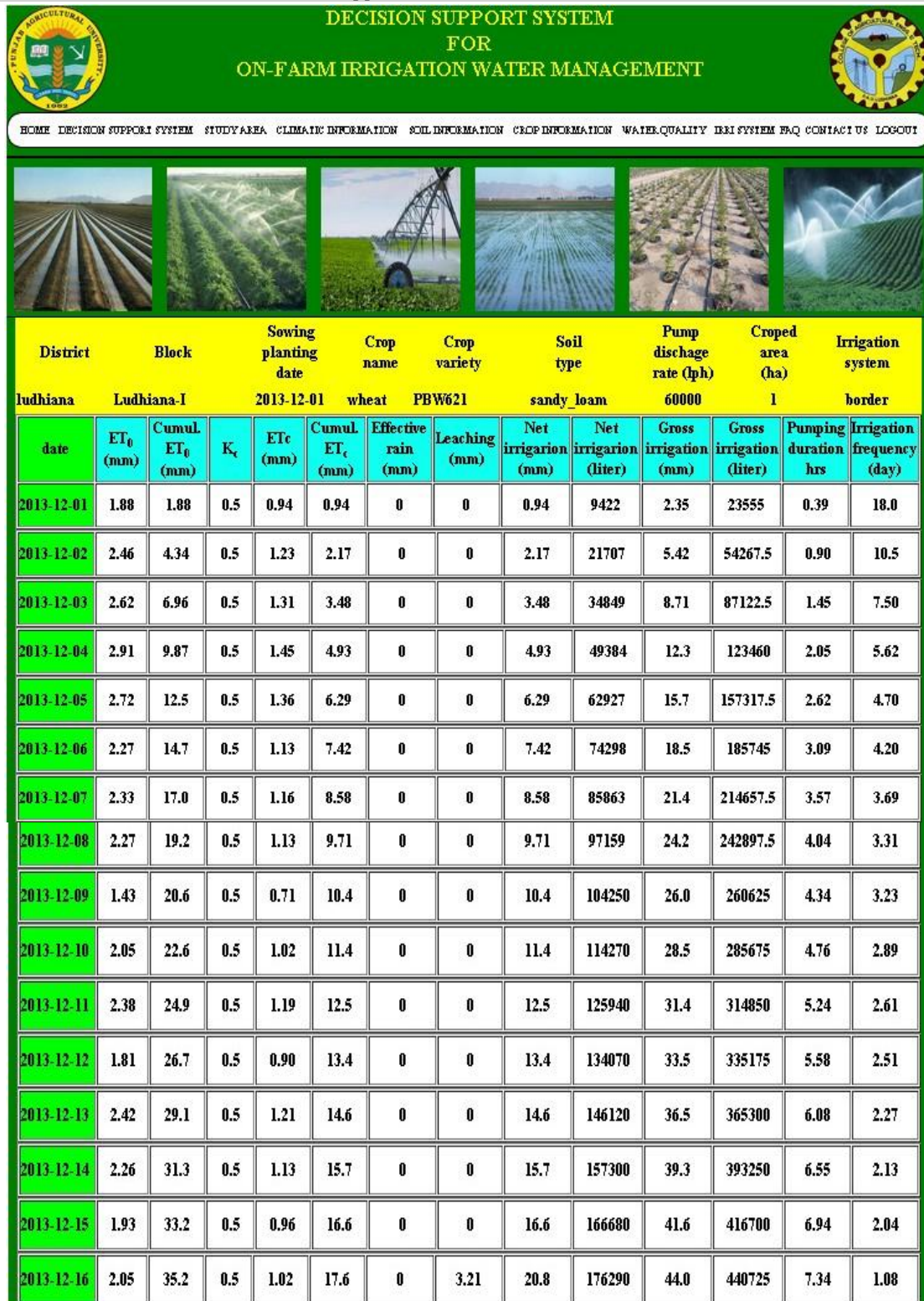
Fig. 16: Output screen of border irrigation system
